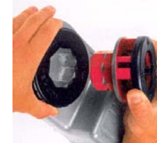
Inserting the die head
